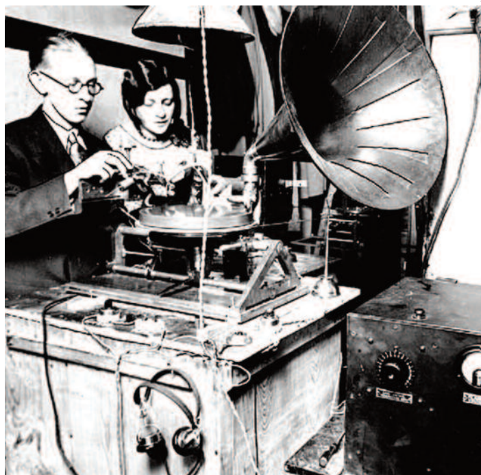
Gennett's portable recording lathe, St. Paul, MN, 1927. Although the masses of wires, headphones give the impression of a fully-electrified system, the drive wire to the falling weight mechanism at the rear can just be discerned. Note the primitive playback facility!
