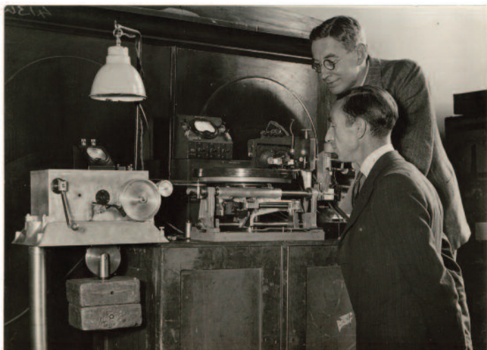
A weight-driven recording lathe as used at HMV in the early 1930s. Note the lead weights and cranking handle to the left.
